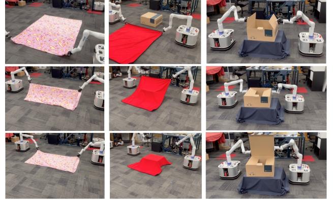
Fig. 10: Qualitative samples of deploying the policy on hardware. We deploy our learned policies to a mobile robot platform to manipulate target objects that are at least 6 times larger than the demonstrated objects. They have different visual appearances, aspect ratios, and physical properties (e.g. friction and elasticity of the cloth) than those in the source tasks. Even with such a large difference between source and target domains, our policy can zero-shot generalize to the target objects and can successfully carry out the task. Please see our website for full videos of these samples.
